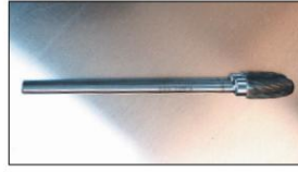
An essential item for port polishing. With just this one tool, you can remove the thickness around the IN and EX ports and valve guides.
