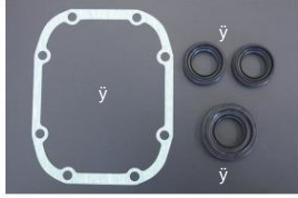
R180 Differential Parts ¥Pinion oil seal ¥900 ¥Side oil seal ¥1,030/ each ¥Diff cover gasket ¥2,180
