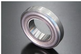
Nissan Clutch Release Bearing Part Number: 40751S ¥1,910 ¥Compatibility (standard) L6 A type FJ20 ¥size D=74.5 d=40 T=19 B¥17 C=62
