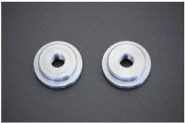
Nissan R180 Bolt Type Conversion Parts - Parts for converting circlip type differentials to bolt type for use on GC10 and S30. Note: Not compatible with Subaru R180. ¥6,000/1SET
