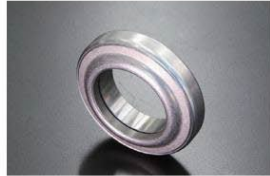
Nissan Clutch Release Bearing Part Number: 4067L1 ¥3,940 *Compatible with OS Twin & Triple (Standard) U20 L4 *size D=67 d=40 T=18.5 B=12.2 C=44
