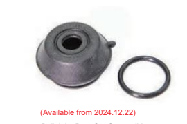
Ball Joint Boot Set Compatible with: S30 Late Model / S10 Late Model (Spindle size: M14) Price: ¥600/set *Individual Boot ¥350, Band ¥250
