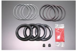
KHC130 Laurel Part number: SP-212 Front caliper seal kit Model year: 1972.4-1975.10 (F disc vehicle) Price: ¥3,350
