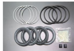
Part number: SP-A25P Front caliper seal kit Compatible with: GC210, GC211 Part number: SP-A25P Price: ¥3,960
