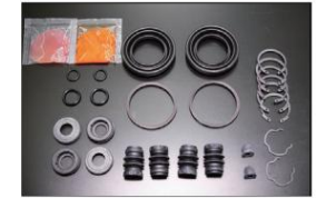
DR30 Turbo (late model) R caliper seal kit Part number: 06P26 Compatible: 1983.2-1985.10 Price: ¥4,400
