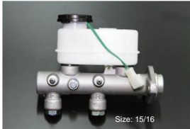
S130 Brake Master Cylinder (for later left-hand drive vehicles) Fits: 81.10-83.8 (L20E) 81.10-83.8 (L28E) Price: ¥42,000
