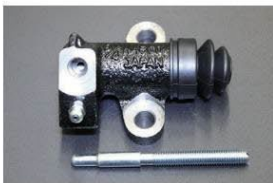
Manual adjustment 3/4 release cylinder Compatible with: GC10/S30 early model Size: 3/4 Price: ¥10,800 (Updated 2026.04.09)
