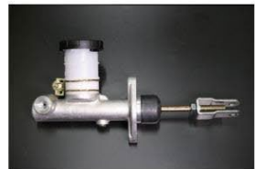
5/8 clutch master cylinder Compatible with: SR311 SP311 Size: 5/8 Price: ¥23,000
