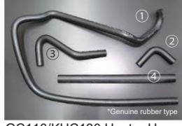
GC110/KHC130 Heater Hose (For early models) *Type where ① and ③ are connected with a heater connector. ① The hose is long, so cut it before use. Price: ¥9,730 /set (Updated 2026.4.16)
