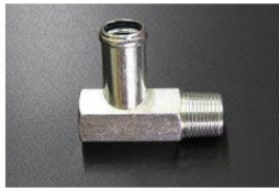
L4 type 16φ-L-shaped head heaterconnector (screw size 3/8, screw diameter 16.6)
