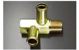
Head heater connector for S130Z (16mm diameter, bifurcated - 1/2 inch screw size, 20.9mm screw diameter) Reproduction Price: ¥6,000
