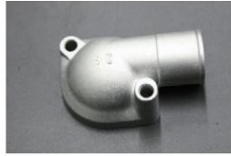
Genuine L-type thermo cover (2 bolts) Fits: L-type Vehicles: S30, GC10, etc. Price: ¥6,080
