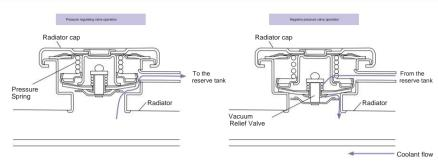
This radiator cap strengthens the pressure valve spring and increases the opening pressure of the radiator.
