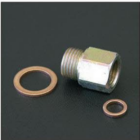
Sensor conversion adapter Product number: P-47W Male M16 x P1.5 - Female M14 x P1.5 Price ¥1,300 Used when mounting an Omori oil temperature gauge with a sensor screw of M14 x P1.5 to a Kameari oil block. It can be installed with a bolt-on as it comes with a washer.
