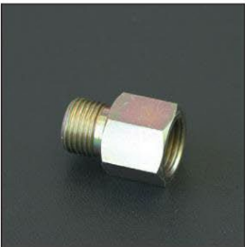
Sensor extension adapter Product number: WT-001BW Male M16 x P1.5 - Female M16 x P1.5 Price ¥1,200 An extension adapter used when the water temperature sensor hits the bottom when installing it in the original position. It comes with washers and can be installed with a bolt-on. Note) A-type engines use inch threads, so please use a special product. Product number: WT-001AW Price: ¥1,200
