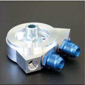
Oil block Product number: E-CONT Compatible with: L-type, 2TG, FJ20 Price ¥15,500 •Oil cooler removal (PF3/8-AN10 for Earls removal) •Oil temperature sensor removal (M16 x P1.5) •Oil pressure sensor removal (PT1/8)
