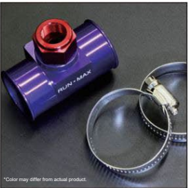
Water temperature gauge hose joint Product number: RW-3616 (for L-type) ¥3,900 Pipe diameter 36φ Sensor M16×P1.5 Product number: RW-3416 (for 2TG) ¥3,900 Pipe diameter 34φ Sensor M16×P1.5 Product number: RW-3216 (4φ) ¥3,900 Pipe diameter 32φ Sensor M16×P1.5 Product number: RW-2816 (for A type) ¥3,900 Pipe diameter 28φ Sensor M16×P1.5 •Put a hose joint between the radiator hoses The mechanical water temperature sensor can be removed.
