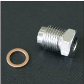
Sensor conversion adapter Product number: P-65W Male M16 x P1.5 - Female PT1/8 Price ¥1,580 Used when mounting an Omori oil temperature gauge with a PT1/8 sensor screw to a Kameari oil block. Comes with a washer and can be bolted on.
