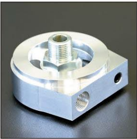
Oil block Product number: NT Compatible with: L-type, FJ20, 2TG Price ¥10,700 •Oil temperature sensor removal (M16 x P1.5) •Oil pressure sensor removal (PT1/8)
