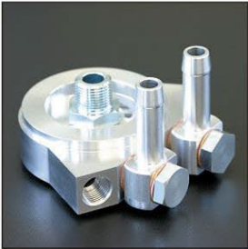
Oil block Product number: CONTL Compatible with: FJ20, L-type, 2TG Price ¥15,500 •Oil cooler removal (PF3/8-φ14.5L-type hose joint) •Oil temperature sensor removal (M16×P1.5) •Oil pressure sensor removal (PT1/8) *By changing the oil element to a smaller diameter, it can be used with FJ20, L-type, and 2TG.
