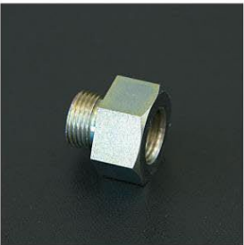
Sensor Drain Adapter Product number: OT-007W Male PF3/8-Female M16×P1.5 Price ¥1,350 Adapter for removing the oil temperature sensor from the oil pan drain cock with 3/8 thread for L-type and A-type. Includes washer. It can be installed with a bolt-on. Depending on the vehicle model and height, attention must be paid to safe ground clearance.
