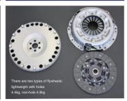
580k cover + reinforced non-asbestos specification
