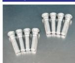
Racing hub bolts that are 15mm longer than the original! Thread length: 35mm Neck length: 50mm Thread pitch: M12 x P1.25 (for Nissan vehicles) Press-fit dimensions (serration): 13mm
