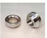
A part that is attached to the top of the rear suspension to raise the vehicle height by approximately 20 mm.
