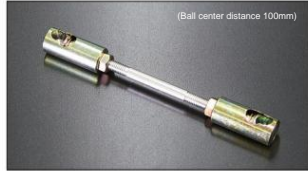
(Ball center distance 100mm) •STD turnbuckle (gold) ¥2,600 The gold part is made of brass, which is resistant to cracking and easy to attach and remove. (Both sides have right-handed threads.)
