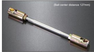
(Ball center distance 127mm) •Long turnbuckle (gold) ¥3,500 Components of the 2TG linkage kit. The gold parts are made of brass, which is resistant to cracking and easy to attach and detach. (Both sides are positive threaded type)
