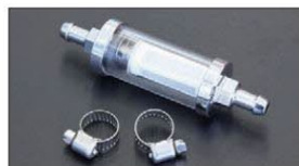
• Fuel filter with magnet ¥4,000 *This glass tube type filter can be disassembled and cleaned, and the magnet inside catches rust and iron filings. (For 8mm hoses. Two hose clamps included.)
