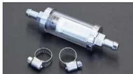
•Fuel filter with magnet Unit ¥4,000 *A glass tube type filter that can be disassembled and cleaned, with a magnet built in to catch rust and iron powder. (For 8 mm hoses. Two hose bands included.)
