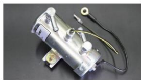
•Mitsuba type fuel pump ¥17,000 *Discharge volume 1.4L/min Maximum discharge pressure 0.3kg/cm2 *Low fuel pressure type exclusively for carburetor vehicles. Fuel regulator can be used without a regulator.
