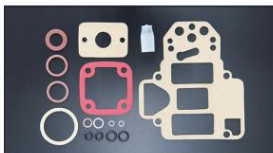
*WEBER Gasket set Unit ¥4,800 *There are different phases depending on the model (image is DCOE9) DCOE9, DCOE151, DCOE152 etc.
