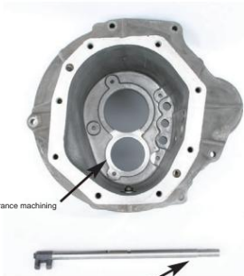
Rod diameter ÿ1.6 is cut to ÿ1.4
