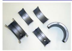
Unlike the general WPC process, molybdenum disulfide powder, which is well known as a solid lubricant, is directly injected. By doing so, the solid lubricant diffuses and penetrates into the metal surface structure, and at the same time, fine irregularities are formed on the surface, enhancing the oil film retention effect. This double effect increases and reduces friction, and reduces the generation of frictional heat. This reduces the seizure load and significantly improves engine damage.
