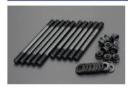
This is a stud type head bolt designed by ARP, an American company. It has a strength standard of 200,000 PSI, and ensures sufficient tensile strength. In addition, the use of stud bolts reduces the deformation of the cylinder bore caused by tightening the head bolts by half, and stabilizes the piston clearance.
