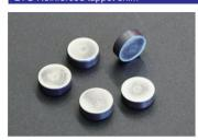
To prevent variation in valve clearance, heat-treated chromium alloy with excellent wear resistance is used. Thickness settings range from 1.3mm to 7.0mm in 0.05mm increments and come in 115 different types.
