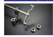
If the ball joint is worn out, the throttle opening will be unstable and no matter how much you adjust the carburetor, the throttle opening will not be synchronized. This ball joint is made of abrasion-resistant num copper and has an oversized design, which stabilizes the throttle linkage shaft runout to within 0.05 mm and allows the carburetor to be synchronized.
