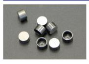
adjusting valve clearance is 2.65mm. When using a cam that has been thinned by machining the stock cam, it is possible to adjust the clearance by placing an outer clearance cap on top of the valve cap.
