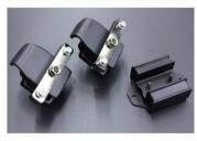
The engine vibrations specific to the FJ20 not only have a egative effect on the engine and carburetor, but also affect the shifting feeling when they are transmitted to the shift lever. This reinforced mount absorbs vibrations appropriately, improves driving stability, and transmits engine power to the drivetrain without loss.
