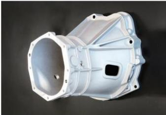
The genuine 71A transmission cannot be repaired because most of the overhaul parts are no longer manufactured. By replacing this housing with a 71B transmission from a GC210 or S130, the 71B can be installed. Furthermore, with some modification it can be changed to a 71C, allowing the combination of a cross transmission or quick shift. (The 71B also has a cross transmission setting.)
