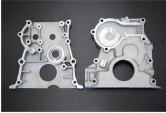
The S20 front cover is a difficult part to repair, as it is prone to corrosion around the water pump and cracks and damage to the driven gear bearing support. This reproduction uses steel for the bearing insertion part. It is designed with an emphasis on durability.
