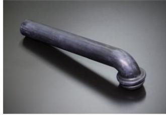
This is a blow-by hose that connects the tappet cover to the air cleaner box. Because it is a rubber product, it needs to be replaced periodically before cracks occur. It is made of flexible oil-resistant rubber.
