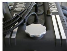
The original shape has been kept intact, with an emphasis on aesthetics achieved by using an all-aluminum buffed finish.
