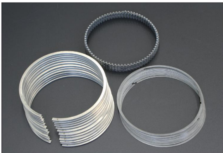
*This ring is a reinforced piston ring that comes standard with the Kameari Piston Kit. It is designed to increase tension and surface pressure appropriately.
