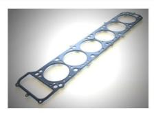
Beads are pressed around the combustion chamber, water holes, and oil holes, where high sealing performance is required. The bead type ensures high surface pressure. The layout is appropriately distributed according to bead width and height.
