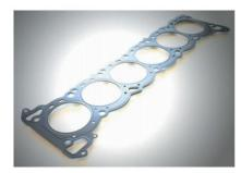
The stopper type was developed to improve the sealing performance around the combustion chamber. The inner plate is wrapped around the bore in a grommet shape, and the stopper part is overlapped with the outer bead plate, improving the sealing performance with a two-stage structure of the stopper and bead.
