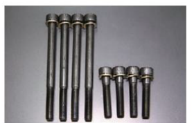
L4 Cam Holder Reinforcement Bolt SET *slightly longer setting to prevent damage to the threads M8x100 Tightening: 2.5kg/m (24.5N·m) M8x40 Tightening: 2.2kg/m (21.5N·m) Price: ¥1,800
