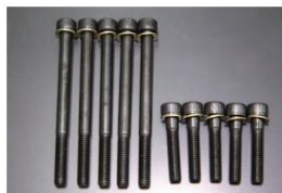
L6 Cam Holder Reinforcement Bolt SET *slightly longer setting to prevent damage to the threads M8x100 Tightening: 2.5kg/m (24.5N·m) M8x40 Tightening: 2.2kg/m (21.5N·m) Price: ¥2,250
