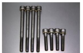
L4 Cam holder reinforced bolt SET * M8x100, slightly longer to prevent damage to the threads Tightening: 2.5kg/m (24.5Nym) M8x40 Tightening: 2.2kg/m (21.5Nym) Price: ¥1,800
