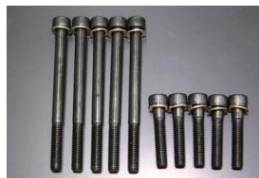
L6 Cam holder reinforcement bolt SET *M8x100, slightly longer setting to prevent damage to the threads Tightening: 2.5kg/m (24.5Nym) M8x40 Tightening: 2.2kg/m (21.5Nym) Price: ¥2,250
