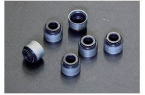
L-type low head valve oil seal ¥280/each A type that is 1.3 mm shorter in height than the genuine part. It increases the clearance before bottoming out, allowing for greater valve lift.
