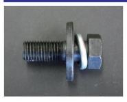
Most camshaft knock pin problems are caused by improper tightening of the center bolt. Using a reinforced bolt reduces the load on the
