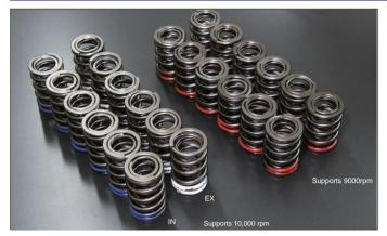
ne natural frequency is improved by using an inner/outer press-fit + unequal pitch. Aiming for instantaneous power and high rotation. KAMEARI know-how is utilized in the calculated load settings.
